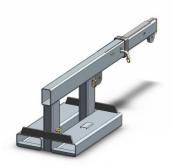
The actual capacity rating of the truck with the jib installed shall be derated to 80% of the calculated capacity to compensate for the dynamic effects of the suspended load.
