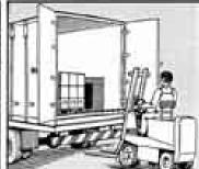
The use of pulling attachments attached to the forks, fork carriage or mast, commonly referred to as pallet puller as shown in *illustration 1* **is not allowed** for the following reasons;
