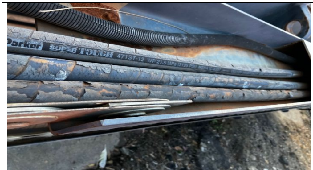
Figure 3 - Damaged hydraulic lines
